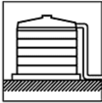
Tank overflow must be piped away from tank to avoid undermining tank base.
